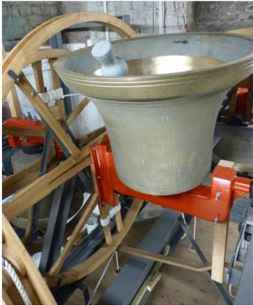
The bells are 'raised' so that the bell mouth faces upwards, and a simple mechanical design allows the bell to rest in this upside-down position. The bell-ringer pulls the rope attached to the wheel, and the bell rotates a complete circle (360°) and the clapper strikes the bell at the end of the revolution.
