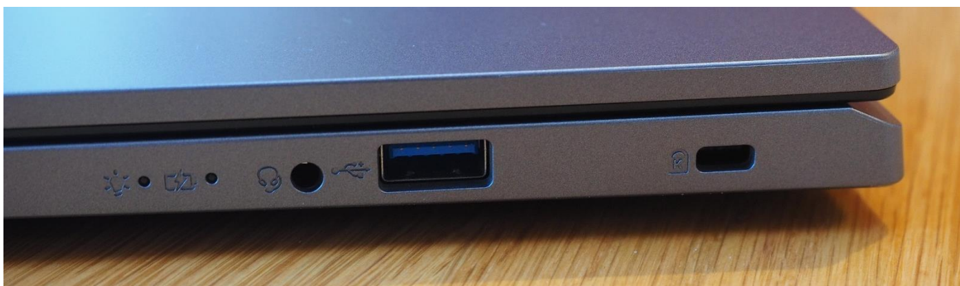
Connection sockets for 3.5mm audio jack (headphones), USB-A, and Kensington lock.
