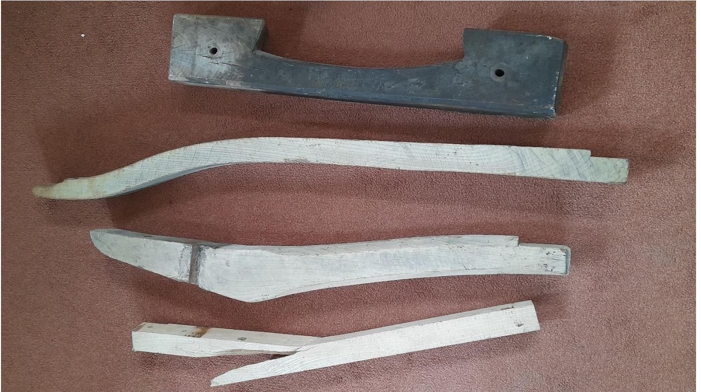
Top = Running Board; Upper Middle = Slider; Lower Middle = Stay; Bottom = Broken Stay
