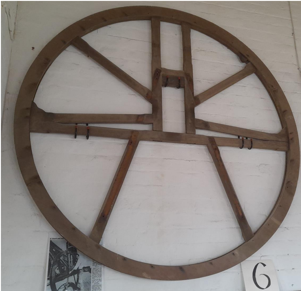
6' (1.8m) Diameter Bell Wheel – Splits into two (flanges at join have to be removed)
