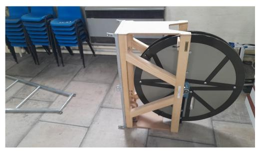
Now match the letters marked on the frame in black marker pen, and attach the appropriate A frame lying flat on the floor to the simulator, finger tight only.
