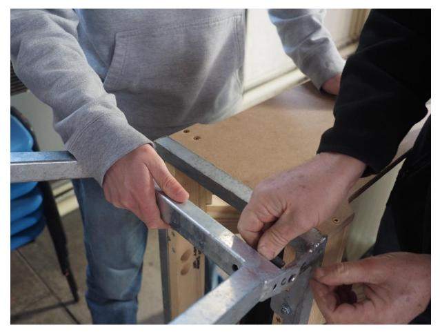
The next step is to attach the cross braces. There are 4 available, but experience tells that the structure (once tightened up) is still rigid with 3 out of the 4, which can provide easier access to members of the public entering the Wombel under supervision, but also to give unimpeded access to the supervising tutor to assist the member of the public with handling the rope.
